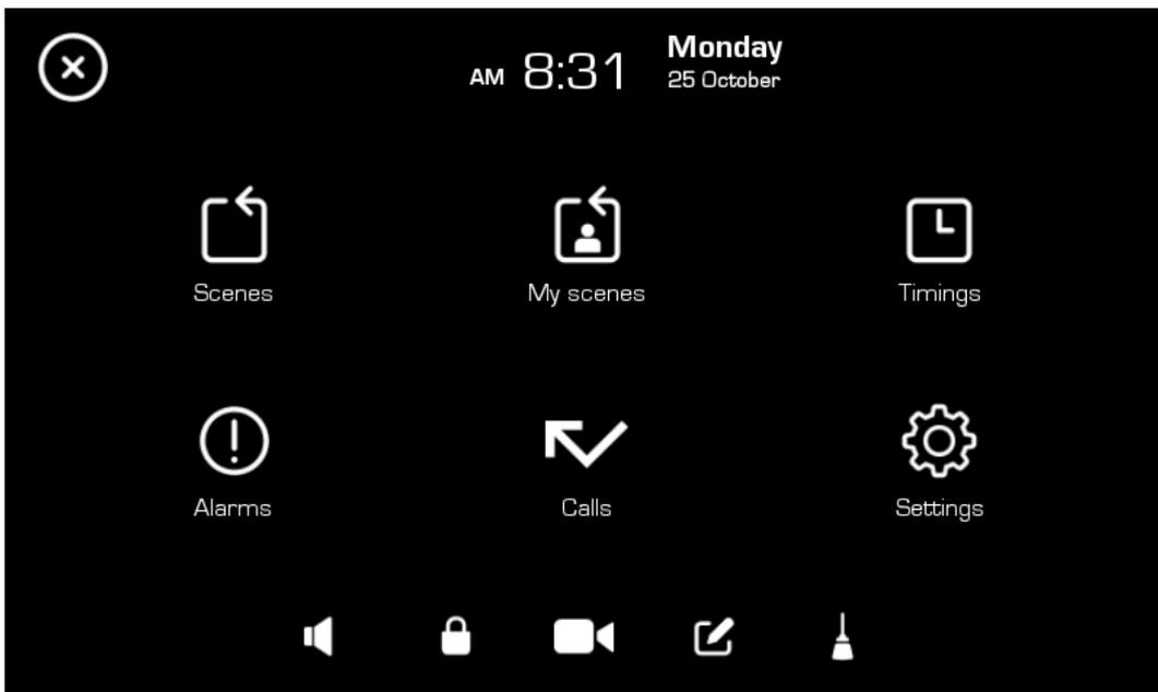
When the alarm status is disarmed, you can click on the icon to execute the arming order, a message will appear "The alarm is being armed" and the icon will flash white and orange. The lock icon will also appear blinking at the top right of the main screen.
