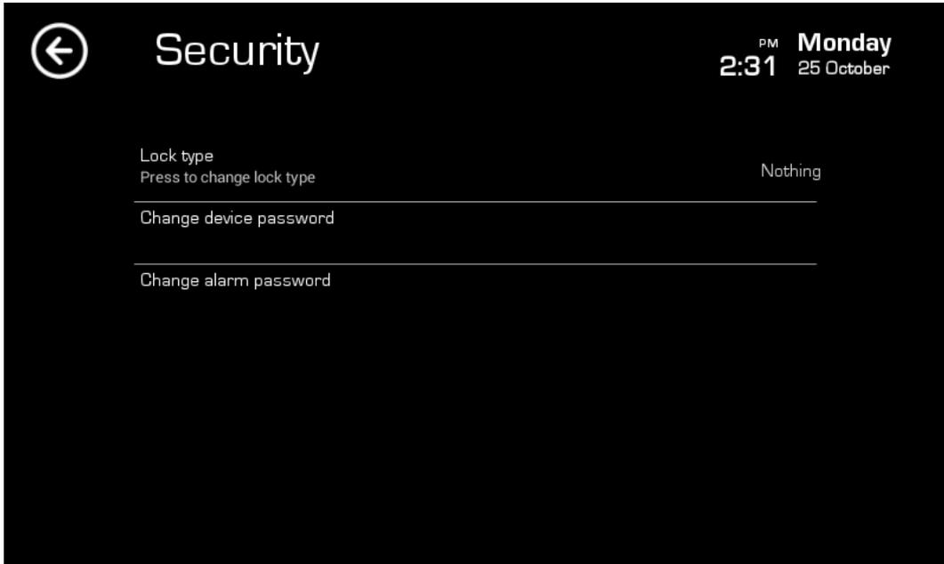
You can change the PIN of the device by clicking on that option. A window opens where you must enter the old password and the one you want to set. The default password is blank.
