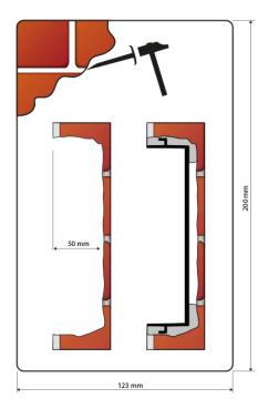
Hole dimensions for flush mounting
