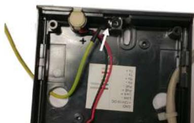
Assemble the set and ground the cable.
