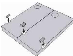
5. Install blank modules on the unused side holes as shown in Figure previous step.
