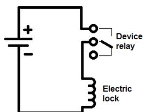
The electric lock is opened by power supply connection.
