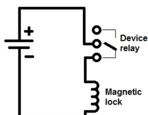
The magnetic lock is opened by power supply disconnection.
