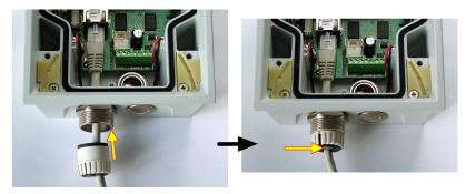
7. Replace and tighten the nut.
