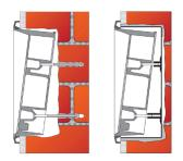
**1.** Make a hole using the template. Suppose that all the required cables have been carried into the hole.
