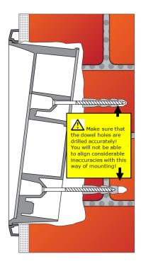
Be sure keep strictly the hole dimensions while mounting the device into classic bricks without the flush mounting box as shown in the figure below.
