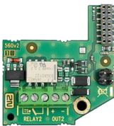
2N IP Force/Safety 2nd relay Additional switching contact for assembly in 2N IP Force/Safety
